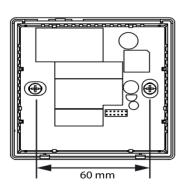
Surface mounting in a 60 mm wall box. Make sure the back cover is in the appropriate position (according to the arrow on it)
