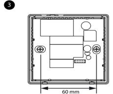
Surface mounting in a 60 mm wall box. Make sure the back cover is in the appropriate position (according to the arrow on it)
