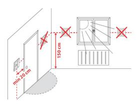
Devices must be mounted on clean, dry indoor place without direct airflow from a heating / cooling device, and not be exposed to dripping or splashing. Before removing the front cover, disconnect the power supply. Wiring, protection and earthing must be installed in compliance with local regulations.
