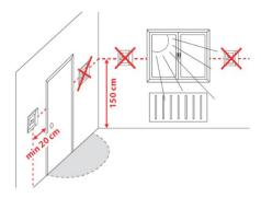
Devices must be mounted on clean, dry indoor place without direct airflow from a heating / cooling device, and not be exposed to dripping or splashing ,Before removing the front cover, disconnect the power supply. Wiring, protection and earthing must be installed in compliance with local regulations.
