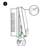
For the convenience of installation, the first step is to wire the volt-free wires, low-voltage wires then high-voltage wires. Check the wires are property connected.
