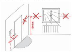
Devices must be mounted on clean, dry indoor place without direct airflow from a heating / cooling device, and not be exposed to dripping or splashing Before removing the front cover, disconnect the power supply. Wiring, protection and earthing must be installed in compliance with local regulations.
