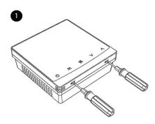
Remove the front cover by prying hooks with flat screw driver at the bottom of the front panel
